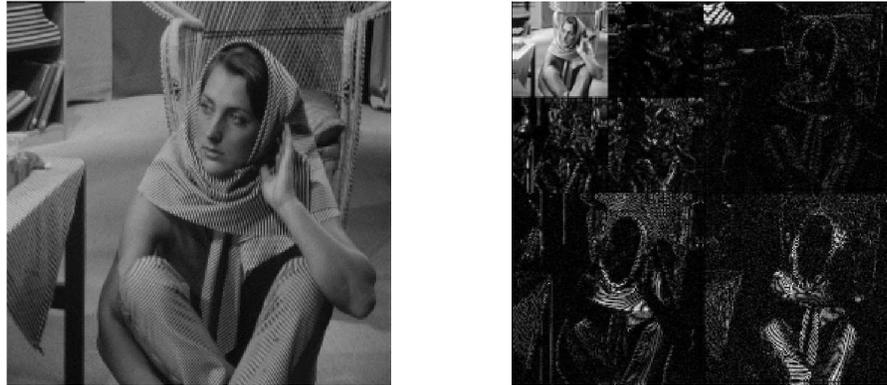
**Figure 2.1:** Left – Sample image of size  $256 \times 256$ . Right – Wavelet decomposition of the sample image containing lot of dark areas which shows that the image is compressible in wavelet domain.
